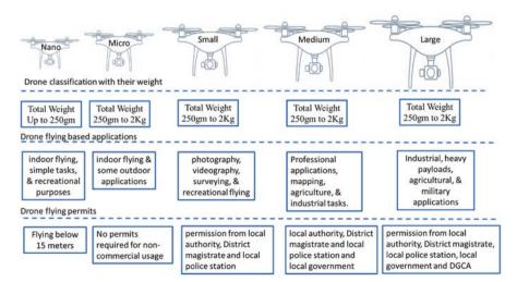
**Fig. 2** Classification of drone based on DGCA, Ministry of Civil Aviation, Government of India (2021): left to right – nano, micro, small, medium, large drones, weight, flying applications, and permits requirements
