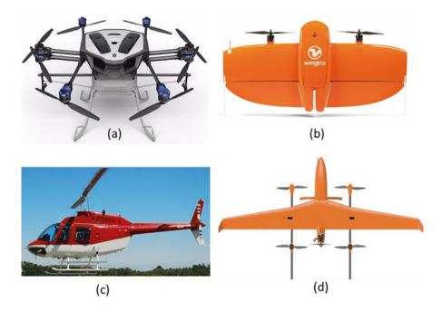
Fig. 1 Types of drone: (a) multi-rotor, (b) fixed-wing, (c) single -wing, and (d) fixed-wing hybrid vertical take-off and landing (VTOL) drones
