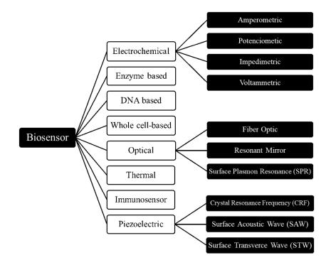
*Figure 4. Classes and sub-classes of biosensors based on the type of transducer (Gieva et al., 2014)*
