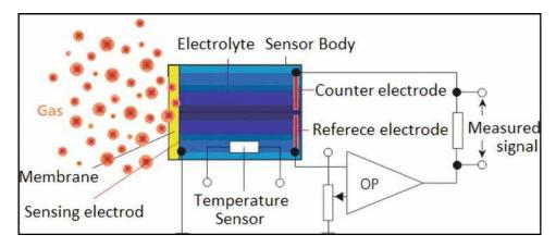
Figure 2. Electrochemical sensor working principal
