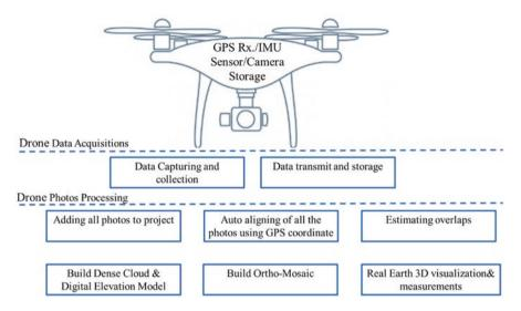
Fig. 3 Drone data acquisition and their processing to get remote sensing data
