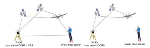
Fig. 4 Drone flying in real-time kinematics (RTK) and post-processing kinematics (PPK) mode of data collection. (Source:ref.: https://www.jouay.com/blog/rtk-drone.html)
